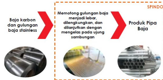
Picture 8. Steel Pipe Production Process
